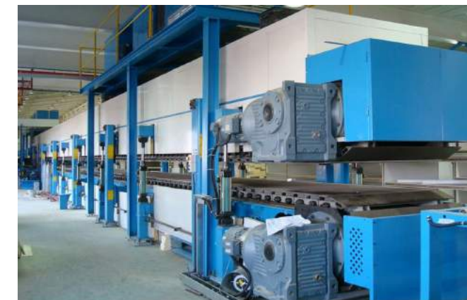
Double belt slat conveyor with main heating system
