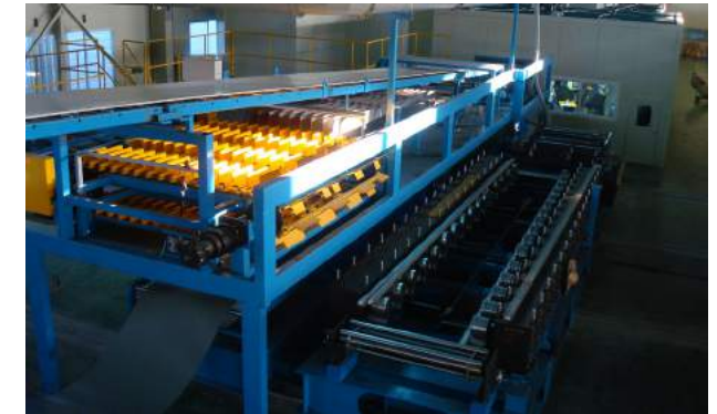
Mineral-wool & PU combined sandwich panel line
