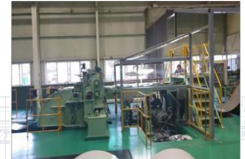
Measuring unit & Rotary shear
