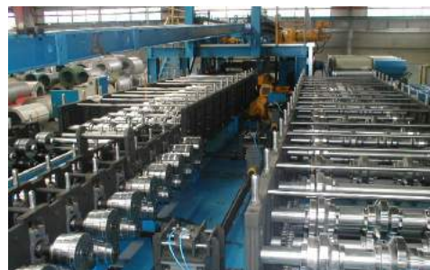
Roll forming machine with press
