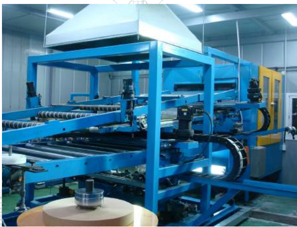
Traverse (Portal) system with side PU injection
