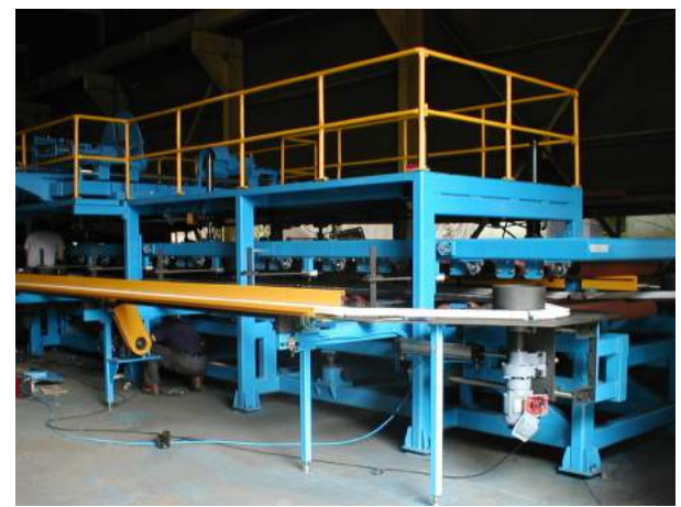
Laminating machine with side guide & block system
