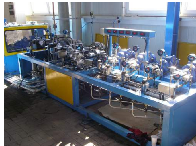
PU/PIR Metering system - 7components with Pentane system
